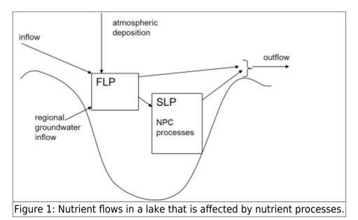
The processes of denitrification, primary production and mineralization have been implemented for both rivers and lakes. For particulate phosphorus (PP) there is an exchange with the river sediments. The rivers dimensions are used in the calculation of these processes. The width and depth of the watercourse are calculated from a number of empirical equations (for more information on these equations see "Modelling phosphorus transport and retention in river networks" by Jörgen Rosberg).
