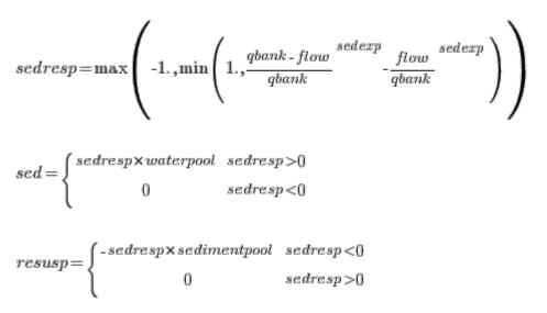
where *flow* is the current river flow (m3/s) and *qbank* is the flow when river is filled to the brim. This flow is calculated as the second largest simulated flow in the last year. It is adjusted with a correction factor of 0.7 before use in the *sedresp* equation.
