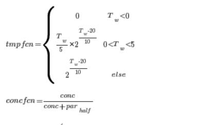
$denitr = MIN \left( 0.5 \times INpool, par_{den} \times area \times concfcn \times tmpfcn \right)$
